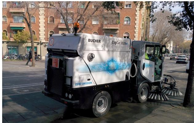
Electric sweeper with capacity of 2 m 3 .
