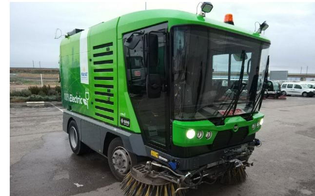
Prototype electric sweeper with capacity of 4/5 m 3 .
