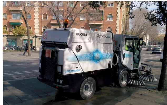
Electric sweeper with capacity of 2 m 3 .
