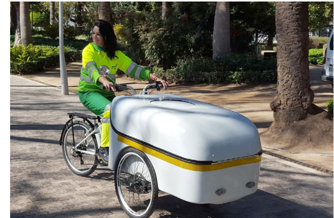
PELUSA assisted pedaling tricycle with auxiliary electric motor.
