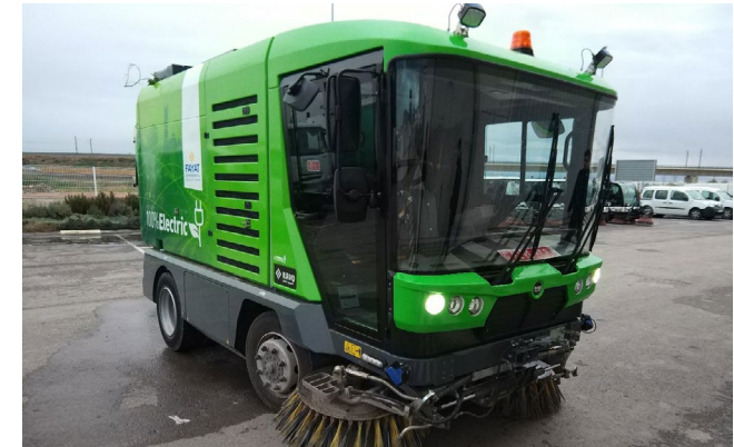
Prototype electric sweeper with capacity of 4/5 m 3 .
