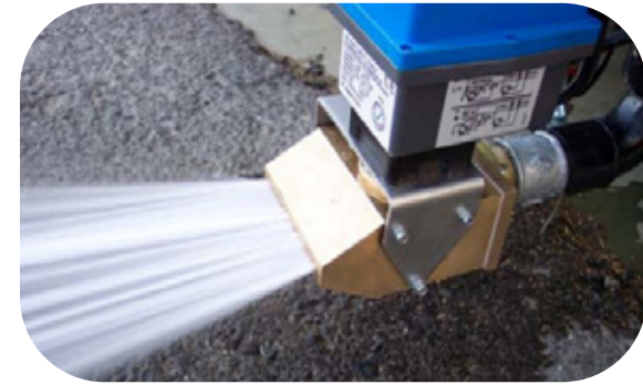
Installation of adjustable bucket dispensers with programmable controllers on the bucket machines
