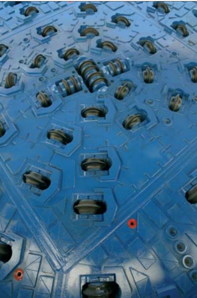
Detail of spinning drill of the TBM-type tunnel boring machine.
